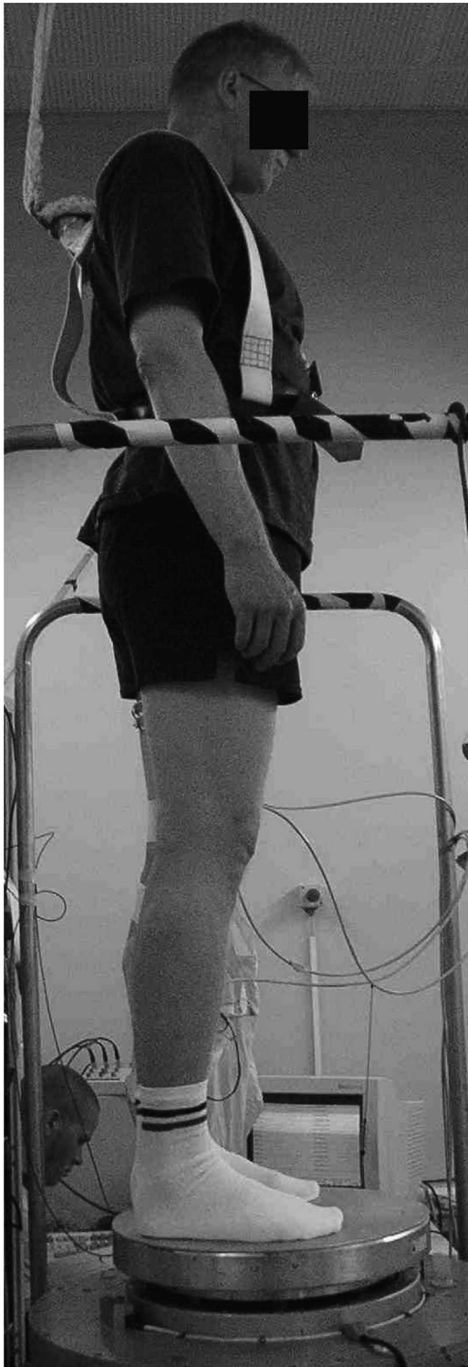
FIG. 1. Vibration system and the typical posture of the subject on the vibration platform.
