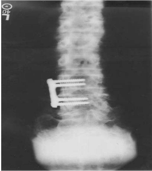
Figure 2. X-ray of a lumbar spine specimen after an anterior lumbar fixation plate was screwed into the L4-5 vertebrae. Note the insertion of two screws per vertebrae.
